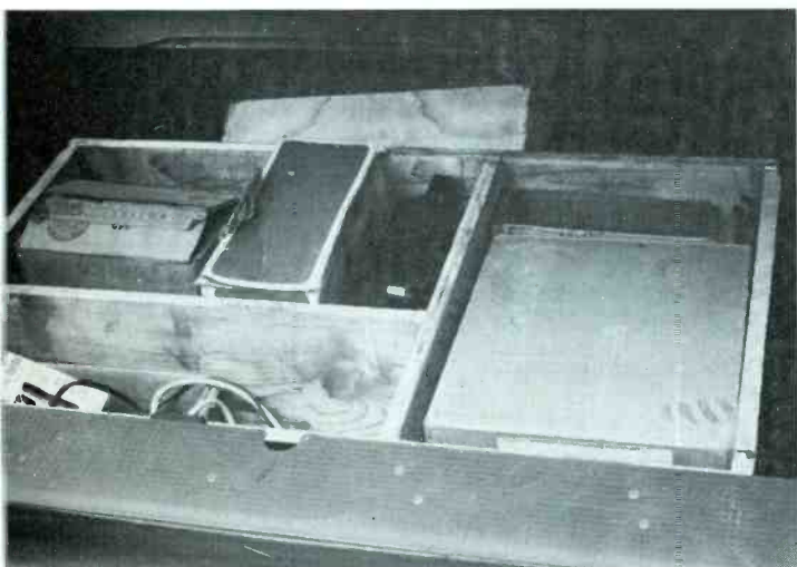
Additional storage space is available in the compartment under the rear flooring. The hidden location offers some protection from thieves and vandals. A wooden box with compartments, built to fit the space, keeps components in order, and gives protection for test equipment.
